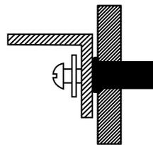
2. The cooler curtain header is placed against the flange of the well-nut. A machine screw (and washer) are used to, engage the threads inside the well-nut.
