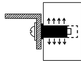
4. In a blind hole, where the wall is solid material, the body of the well-nut expands tightly against the walls of the hole. This produces a secure dependable anchor.
