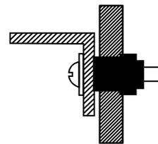
3. As the machine screw is tightened, the well-nut's neoprene body is compressed and expanded, forming an anchor against the inner surface of the wall.
